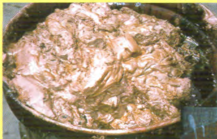
Centrifugally removed copper and aluminum fines
